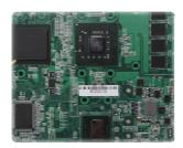
Axiomtek tBOX320 adopts an onboard processor and onboard DRAM which greatly reduces the impact of vibration and shock ideally for railway fields. To prevent ESD and over-voltage, this compact-size system is equipped with 4 isolated RS-232/422/485 ports and 1 isolated digital I/O connector for offering excellent power protection.
